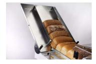
Optional chute for extra bread infeed storage for up to 15 breads. Chute with side guide strips for different seizes of bread and can be folded down completely when not in use.
